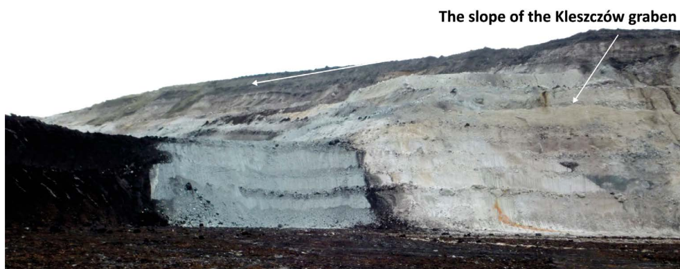
Fig. 1. Bełchatów lignite mine, the Szczerców exploitation field. Exposure of the limestone floor at the IVth exploitation level, in the ordinate range of +112/+81 m above sea level
